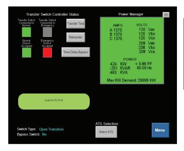
Whereas competitive simulators may utilize computer modeling, the 4000 Switchgear Simulator includes the same color touch screen as the PCS switchgear as well as a PLC to execute the actual sequence of operation from the PCS switchgear.
