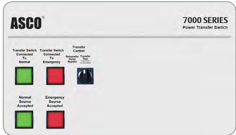
Fig. 16: 7000 SERIES User Controls and Indicators.
