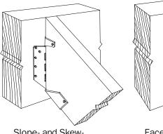
Slope- and Skew-Adjustable Joist Hanger
