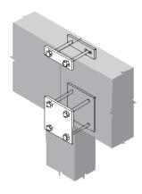
Notched beam bearing. Depth limitations sometimes cause detailing difficulties at the beam supports. A simple solution is to notch the beam at the bearing. This induces large tension perpendicular to grain stresses and leads to splitting of the beam at the root of the notch.
