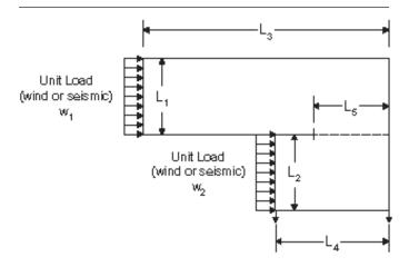
Unit shear along  $L_3 = \frac{W_1 L_1}{2L_3}$
