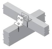
19. Special detail to connect the ridge purlin to sloped members or to the peak of arch members.
