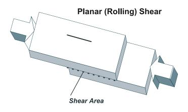
Table M9.2-3 Wood Structural Panel Planar (Rolling) Shear Capacities
