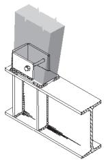
27. Similar to detail 25. This more rigid connection is suitable for spans where arch rotation at the base is small enough to not require the rotational movement permitted in detail 25. Note that, although the shoe is "boxed" a weep slot is provided at the inside face.
