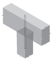
5. Concealed connection in which a steel plate is inserted into a kerf in both the beam and the column. Transverse pins or bolts complete the connection.
