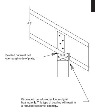
For the high end support, bottom flange bearing in a suitable connector or on a beveled plate is recommended. When slopes exceed 30°, straps or gussets may be needed to resist the tangential component of the reaction.
