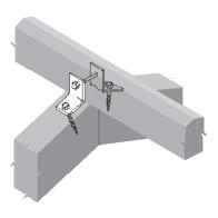
20A. Similar to detail 19, but with the segments of the ridge purlin set flush with the other framing.
