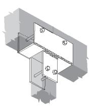
7. Combinations of steel angles and straps, bolted and screwed, to transfer forces.
