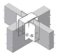
14. Face-mounted hangers are commonly used in beam to beam connections. In a "cross" junction special attention is required to fastener penetration length into the carrying beam (to avoid interference from other side).
