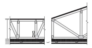
Figure M16.1-22 Cross Sections of Possible One-Hour Area Separations
