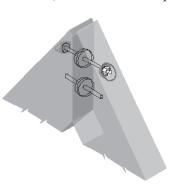
24. Similar to detail 22 for low slope arches. Side plates replace the threaded rod.
