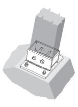
28. For very long spans or other cases where large rotations must be accommodated, a true hinge connection may be required.
