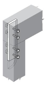
6. Custom welded column caps can be designed to transfer shear, uplift, and splice forces. Note design variations to provide sufficient bearing area for each of the beams and differing plate widths to accommodate differences between the column and the beam widths.
