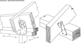
Seismic and Hurricane Ties Connecting Roof Framing to Top Plates
