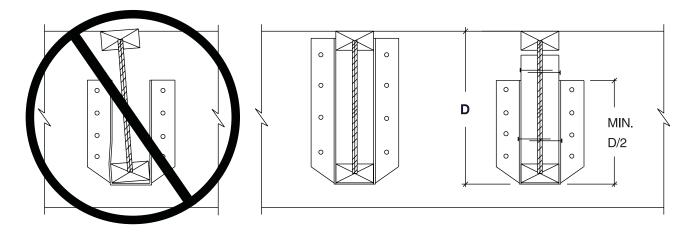
Top and bottom joist flanges must be laterally restrained against rotation.
