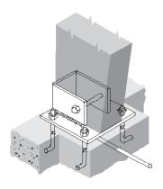
26. Arch base fastened directly to a steel tie beam in a shoe-type connection.
