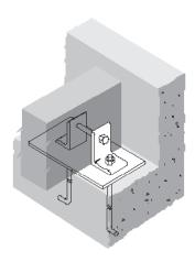
2. Similar to detail 1 with a steel bearing plate only under the beam.
