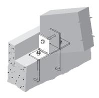
Hanging to underside of beam. Sometimes it is advantageous to hang a load from the underside of a beam. This is acceptable as long as the hanger is fastened to the upper half of the beam. Fastening to the lower half of the beam may induce splits.
