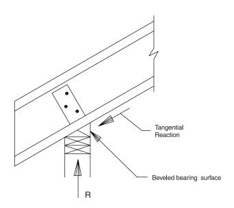
Tangential reactions may exceed a standard 2 nail connection capacity on steep slopes (above 20 to 30 degrees.)
