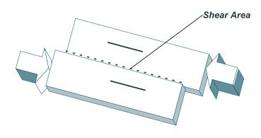
Figure M9.2-4 Planar (Rolling) Shear or Shear-in-the-Plane for Wood Structural Panels
