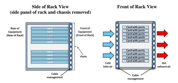
Note how the cards are oriented horizontally and the side to side cooling air flow stream travels parallel to the cards.
