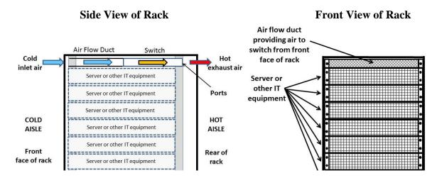
This can be achieved by a combination of a switch that has front to rear air flow and duct work that extends the switch to the front face of the rack.
