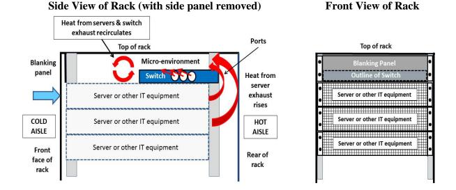
Fig. 11 Small 1U form factor switch mounted behind a blanking panel.
