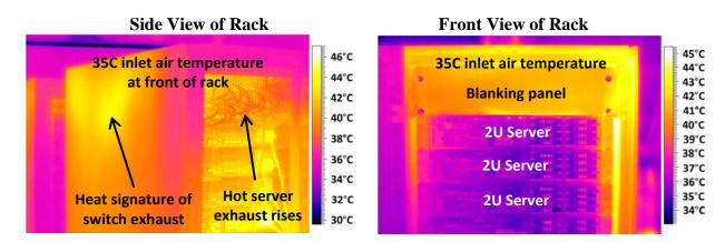
Fig. 12 Infrared images of switch installed behind a blanking panel.
