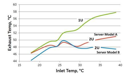
With an inlet temperature of 27°C, which is still within the ASHRAE recommended range, the exhaust temperature can reach 52°C, which is above the maximum temperature rating of many small form factor switches.
