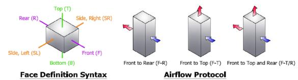
Fig. 6 ASHRAE standard nomenclature for air flow paths through server equipment [13]
