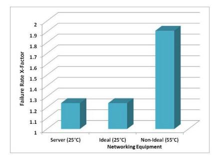
Fig. 19 X-factor failure rate comparison of servers and networking equipment.
