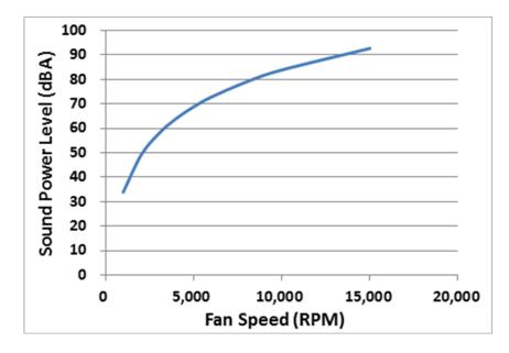
Fig. 21 Example of fan sound power as a function of fan speed.
