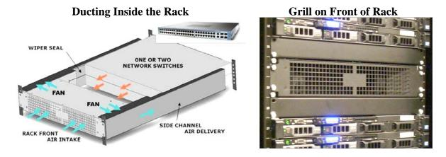
Fig. 20 Example of commercially available fan assisted duct work.
