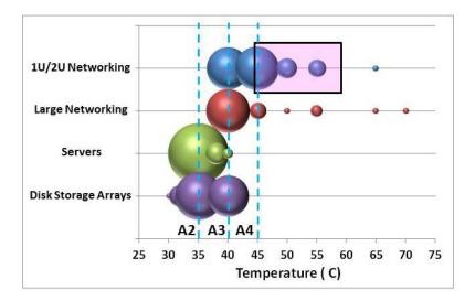
Fig. 17 Server exhaust temperature range super-imposed on benchmarking data.
