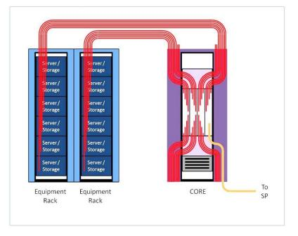
Fig. 2 Example of a simple network implementation typical of a small data center.
