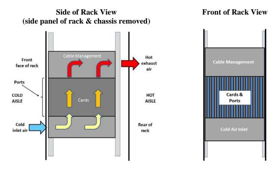
Fig. 7A Large switch, typically full and half size rack, with front to rear air flow.
