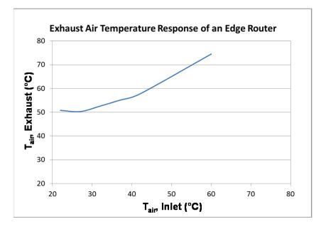
Note at 20°C inlet the air temperature rise is nearly 30°C whereas for an air inlet temperature of 60°C the air temperature rise is closer to 15°C. At 60°C the fans are running at high speed and moving much more air than at 20°C.
