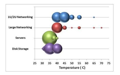
Fig. 5 Maximum temperature rating benchmarking survey results.
