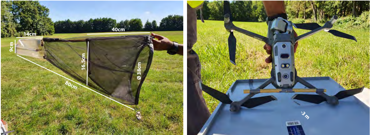
Figure 2. Hanging net specifications (left) – Mavic Pro with cane and fishing line (3 m) attached to net (right) © Shahrukh Kamran
