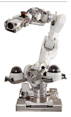
monitoring of ceilings and other inaccessible locations. Although the purpose of the robot was altered and many specification changes were made along the way, High-Access Survey Robot was completed in June 2013 (Fig. 35). This robot had the capability to perform detailed survey tasks under remote control even in the complexity of structure inside a nuclear reactor building. The robot was twice sent into the Fukushima Daiichi Nuclear Power Station, and it performed survey tasks successfully.
