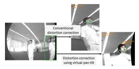
Fig. 24 Correction of image distortion
