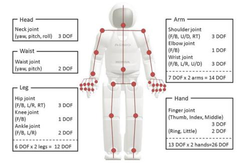
Fig. 25 Joint configuration and DOF (degree of freedom)
