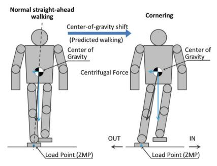
Fig. 12 Center-of-gravity shift
