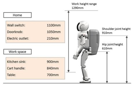
Fig. 11 Investigation of robot dimension
