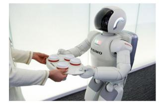
For example, in handing over a tray, the eye camera installed in the robot's head and force sensors in the wrists are used. The camera and the sensors detect the movement of the tray so that the robot can match its actions to the other party and hand over the tray without fail (Fig. 17).
