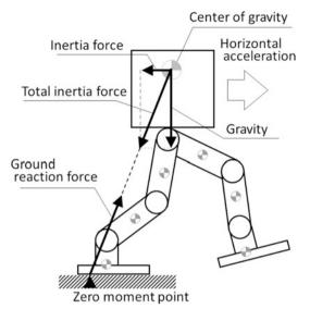
This is accomplished by actively changing the robot's stride length or center of gravity.
