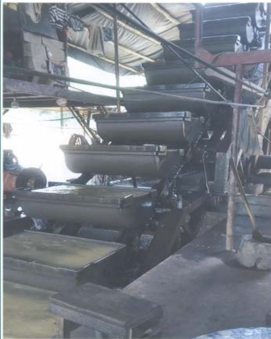
Figure 8. A mechanical conveyer for scooping the river bed for gold.
