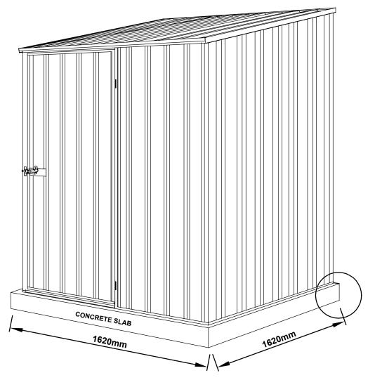
For construction in non-cyclonic areas Wind rating: N2 as per AS4055-2012
