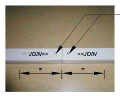
Finished Channel. The joined channels should now look like the picture with the CSJ positioned equally inside of the joined channels. Drill out holes with 3mm drill bit in CSJ to match the holes in channel and secure with the screws supplied. These may have to be temporarily removed during assembly.
