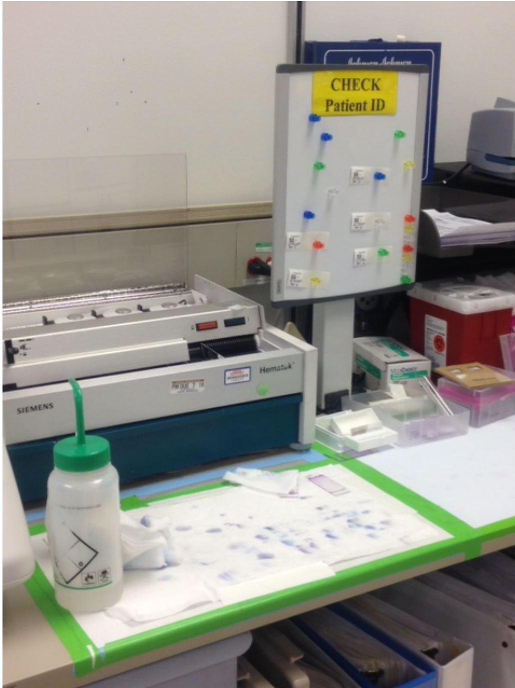
Color-coded magnetic board – holds slide labels to affix to pencil-marked slides after staining; keeps them sorted and separated and prevents loss
