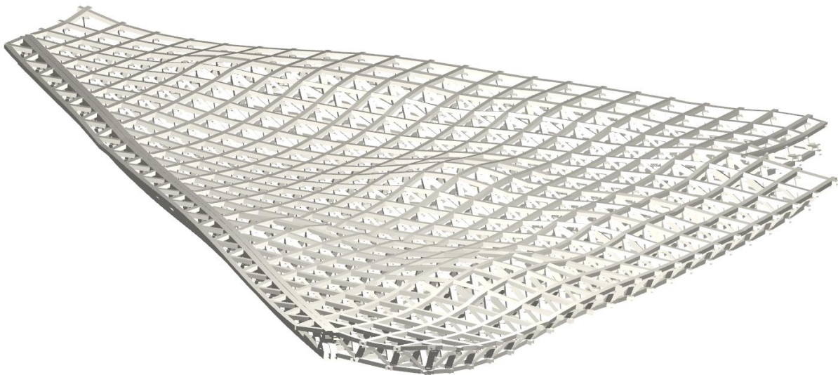
Figure 11: Exaggerated deflected shape of the structural model
