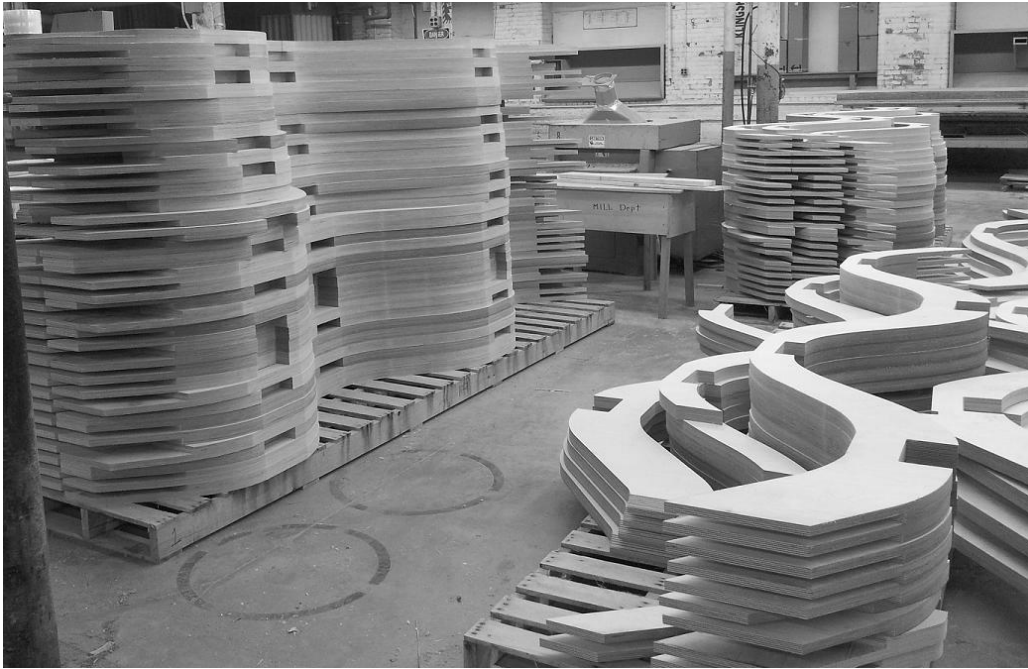
Figure 12: Web laminations after cutting
