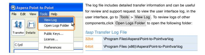
The logs folder contains files of specific components. Older logs are stored in the same file name with incremental number attached, such as *ascmd.0.log*.
