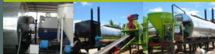
* INTERNAL WIRING WITH JUNCTION BOX & BITUMEN TANK WITH LIME FILLER + LDO TANK
