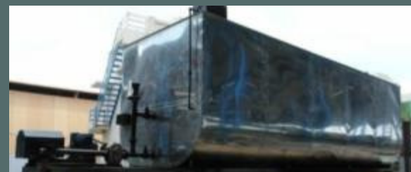
"U" SHAPED BITUMEN TANK
