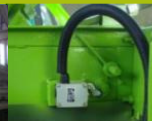
NO FLOW INDICATOR SWITCH
