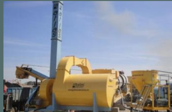
WET DUST COLLECTOR POLLUTION CONTROL UNIT WITH CHIMNEY
