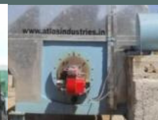
BITUMEN TANK BURNER
