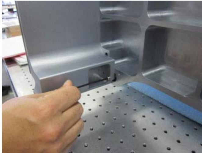
Figure Bottom screw located at outer hole
