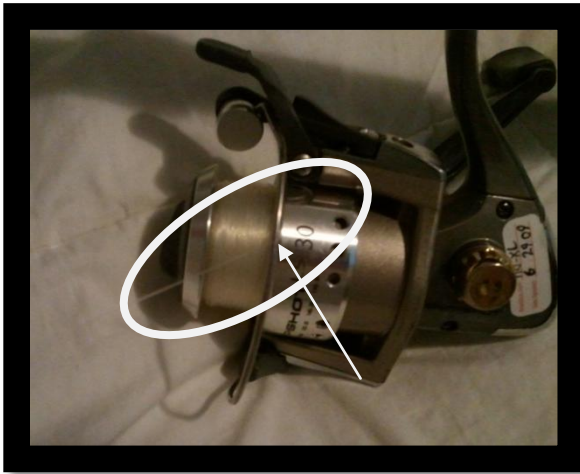
Figure 5.1: Pull the line around the outside of the bail.
