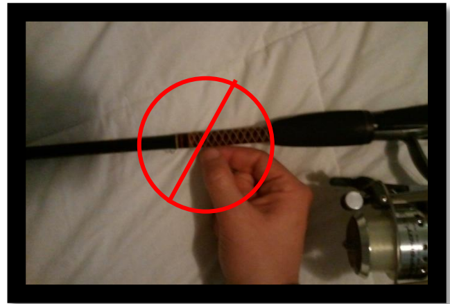
Figure 5.2: DO NOT PULL THE LINE THROUGH THE HOOK KEEPER (THE VERY SMALL HOLE CLOSEST TO THE REEL AND HANDLE).
