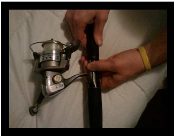
Figure 3.3: Twist the screwing mechanism of the handle over the opposite edge of the reel foot.
