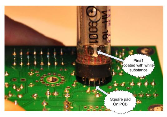
Pin #1 and footprint verification before soldering
