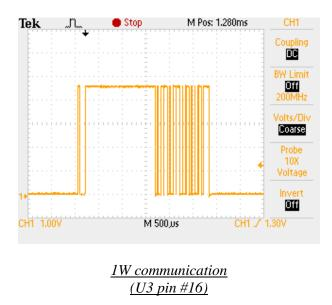
Note clock must be set to the temperature readout state in order to look for 1W communication on the bus. Column separator signal go through repeater on Q1 transistor because it switches high voltage bulb.
