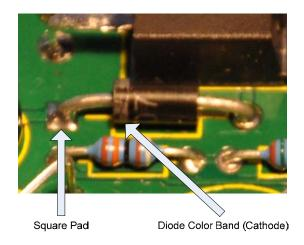
UF4007 diode placing
