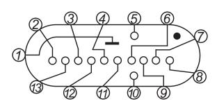
Pin numbering starts clockwise from the first pin, which is labeled on the component capsule by an arrow. The pin numbering scheme above is valid when the component is observed from the bottom.
