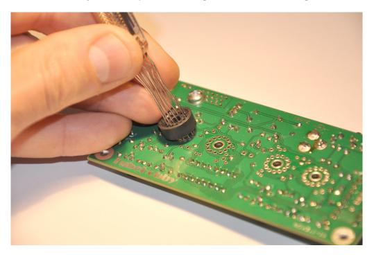
Insert nixie tube at the angle holding spacer near the end of wires
