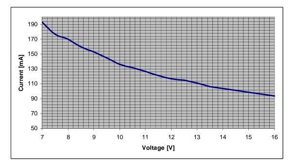
Graph below shows current consumption according to power supply voltage. Tubes' voltage set to 170V. Backlight enabled at full intensity.
