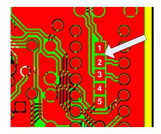
Programming connector has etched jumper between pin #1 and pin #2
