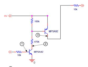
NOTE X Waveforms on these points are provided. Number means oscope channel.
