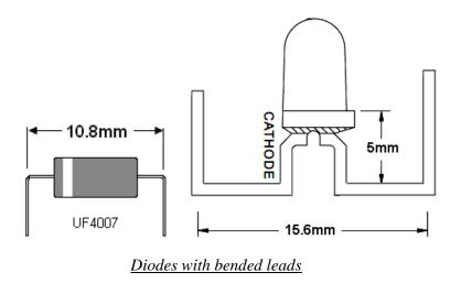
Take the **UF4007** diode and install it into clock board at the location **D1**. Ensure that the direction of the diode matches the silk screen outline on clock board. Solder it into place and clip off the excess lead length.
