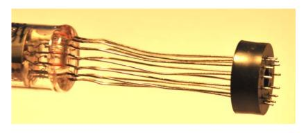
Placing spacer near the end of wires
