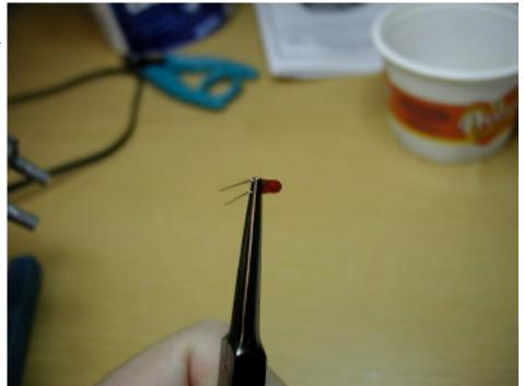
Be sure that the LED can fit through the hole in the frontof the unit before proceeding.
