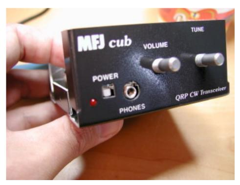
This completes the installation of all the parts which feed through the front of the radio.
