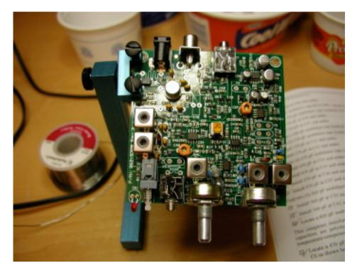
The inductors are next. Two of the inductors look like big resistors. These are placed on the board in the upper left quadrant. Lay the part on the board to see how the leads must be bent to feed through the holes. Pre-bend the leads before you insert the parts.
