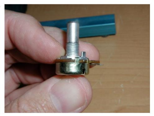
Carefully use diagonal cutters to snip off this tab.
