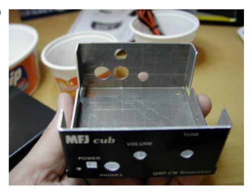
The top slips over the bottom when construction is complete. Notice the hole in the middle of the lid. This allows easy access to the RF power gain potentiometer that is mounted on the board so you can adjust the power later without needing to disassemble the unit.
