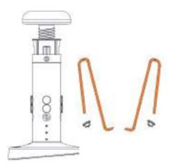
Pull out broken bands and remove plugs from bands.
