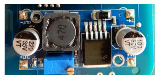
Solder the pins and remove the Buck Converter. When re-fitting, make sure that you have the buck converter the correct way around, 12V 'IN' towards the outer edge of the PCB.
