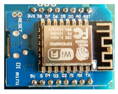
Now remove the Wemos and insert the two sockets headers (that were supplied with the WeMos) into the underside of the PCB and then plug the WeMos in to these headers. The purpose of plugging the WeMos in at this stage is to help get the socket headers straight.
