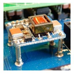
NCH8200HV when mounted on the top of the board
