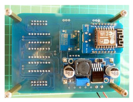
Connect 1 or more LED's to the header on the PCB. These LED's require 5V, GND and Data In to operate. Connect the 'data in' of subsequent LED's to the 'data out' of the previous one.
