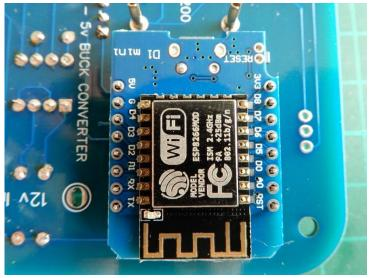
Take care to orient the WeMos correctly so that the pins get soldered to the correct side!
