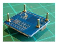
Add the 4 x socket pins for the NCH8200HV power supply, do this by first soldering the 4 pins that came with the power supply to the power supply itself.
