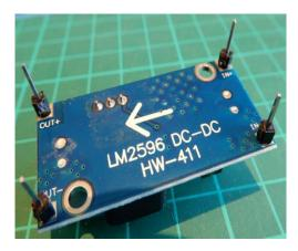
Mount the Buck Converter on the underside of the PCB taking care to mount it the right way around the solder in to place from the top side of the PCB.
