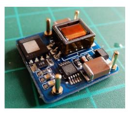
If mounting the NCH8200HV on the top of the main board then mount the pins on the underside of the NCH8200HV.
