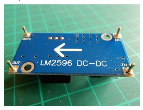
Push 4  $\times$  socket pins on to the pins that you just soldered and push the complete assembly in to the PCB from the Underside.
