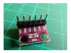
Turn the board over and solder the following components:
