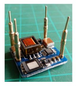
Remove the power supply and trim the short ends of the socket pins on the other side of the board.
