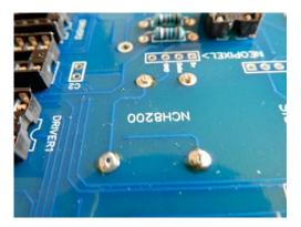
Mounting pins cut off after soldering (NCH8200HV mounted on bottom of board)
