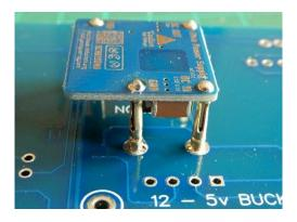
NCH8200HV mounted on the bottom of the board
