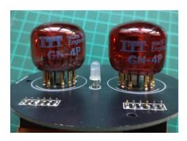
For each board type, mount the socket pins and single RBG LED on the 'top' of the board.
