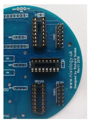
This shows the socket arrangement on the round version of the clock PCB
