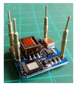
Remove the power supply and trim the short ends of the socket pins on the top side of the board.
