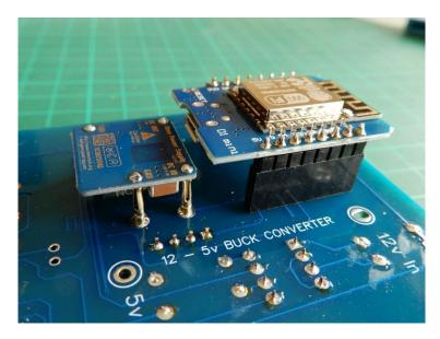
Turn the board over and solder the sockets in to place.
