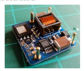
Add the 4 x socket pins for the NCH8200HV power supply, do this by first soldering the 4 pins that came with the power supply to the power supply itself.
