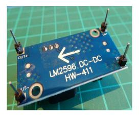
Mount the Buck Converter on the underside of the PCB taking care to mount it the right way around the solder in to place from the top side of the PCB.
