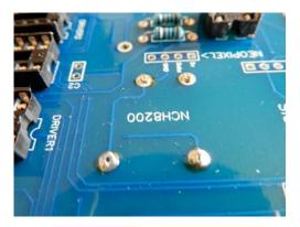
Mounting pins cut off after soldering
