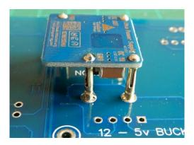
NCH8200HV mounted in position on the bottom of the board.
