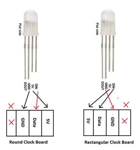
Both images are shown when viewing the neopixel socket with the tube connectors to the right hand side of the neopixel socket.
