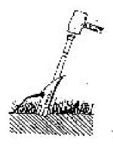
**Step 2**. Wrap the cable three times around the driving rod and pull upward to the anchor in place.
