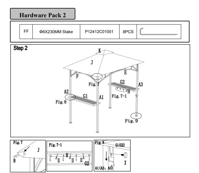
**Fig.7:** Extend the Big Canopy (J) onto the big top by fixing the canopy at four corners of Big Beam (B). **Fig.7-1**: Attach the hook rack (H) to panel 2(G2) with the bolt 2 (II).
