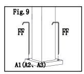
Fig.9: Fix the gazebo to the lawn by using the Stake (FF).
