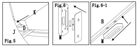
**Fig.5:** Extend the small canopy (K) onto the small top by fixing the canopy at four corners of Small Beam (D). **Fig.6:** Take off the back cover of LED light (M), and match 3 pieces AAA batteries into sockets. Attach back cover to LED light (M). Note: Batteries are not included.
