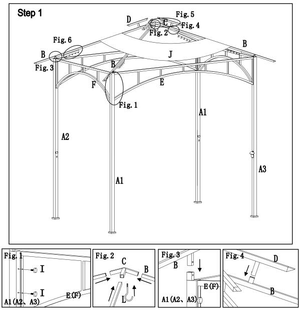
**Fig.1:** Attach the long screen (E) and the short screen (F) to post (A1,A2,A3) with the bolts 1 (I). **Fig.2:** Attach the big beam (B) to the big connector (C), then assemble the hook (L) to the big connector (C). **Fig.3:** Insert the lower connector tube of the big beam (B) into the upper tube of post (A1,A2,A3), then place the big canopy (J) on big top, do not fully spread.
