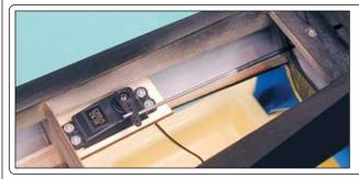
□ Install your rudder servos into the servo trays. Notice the position of the servo output shafts. They should be toward the back of the fuselage.
