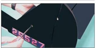
□ Bolt the stabilizer to the fuselage boom, using one long machine screw provided.
