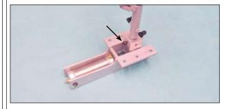
□ Install the nose gear strut into the retract, making sure that the strut is pushed down firmly. Tighten the large socket-cap screw against the strut, then back it off 1/4 of a turn. The strut should be held in place securely, yet be able to rotate smoothly.
