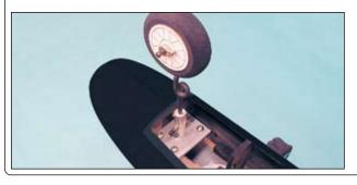
□ Install the nose gear onto the nose gear mounting rails in the center fuselage pod, using the four large wood screws provided. The front edge of the nose gear mounting base should be pushed up against the forward bulkhead.
