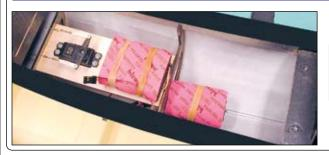
□ Install your battery, receiver and switch into the center fuselage pod.
