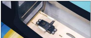
□ Install your steering servo into the servo tray. Notice the position of the servo output shaft. It should be toward the back of the fuselage.
