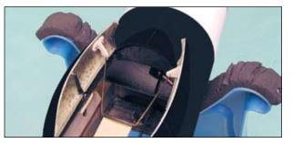
□ Hook the outer hole in each actuator horn over the wire brackets and install the actuator horn onto the landing gear doors, using epoxy and the eight wood screws provided. Position the center of each actuator horn 5/8" (16mm) in front of the back edge and 3/4" (19mm) below the outer edge of the landing gear doors. Angle the actuator horns slightly to line up with the angle of the wire brackets.
