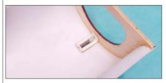
□ The hatch cover is held in place using two hatch latches - one centered at the front and one centered at the back. Install them by cutting
