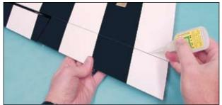
□ Hinge the ailerons to the wing panels, using the six C/A-style hinges provided and a generous amount of thin C/A. Make sure that the tip of each aileron is even with the wing tip and that the hinge gap is as tight as possible to prevent flutter.
