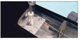
□ Cut the length of pull-pull cable in half and secure one end of each cable to each of the steering couplers, using two of the crimp collets provided.
