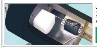
□ Install the fuel tanks, making sure that the tops of the fuel tanks are toward the tops of the fuselage booms. The front of each fuel tank should fit firmly in the predrilled hole in the firewalls and the back of each fuel tank should be angled down enough to clear the wing when it's mounted.
