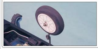
□ Install the wheels, using the two wheel collars and two machine screws provided.
