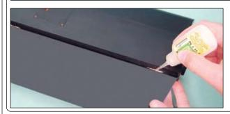
□ Hinge the elevator to the stabilizer, using the four C/A-style hinges provided and a generous amount of thin C/A. Make sure that the elevator is centered between the tips of the stabilizer and that the hinge gap is as tight as possible to prevent flutter.
