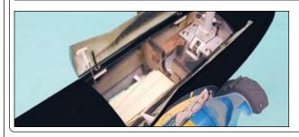
□ Hinge the nose landing gear doors and install the actuator, using the same techniques that you used to install the main landing gear doors and actuators. There are only a few differences: Position each hinge 1" (25mm) in from the front and rear edges of the landing gear doors and install the actuator assembly so that it's hinged from the top, not the bottom, like on the main gear actuators. The bottom of the plywood plate should be even with the bottom of the U-Shaped cutout in the bulkhead.
