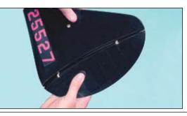
□ Hinge one rudder to each fuselage boom, using two plastic hinge points and 5 minute epoxy. Make sure to push the hinges' pivot points completely into the notch in the rudder to ensure a tight hinge gap.
