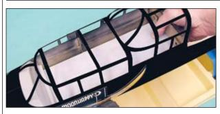
□ Fit and glue the plywood cockpit deck into the slots in the three forward bulkheads. When positioned properly, the back edge of the cockpit deck should be flush with the back of the rear-most bulkhead (wing mounting bulkhead).
