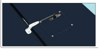
□ Install the servo hatch cover, using the four small wood screws provided.
