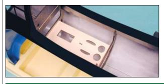
□ Fit and glue the plywood servo tray into the slot in the forward and center bulkheads.
