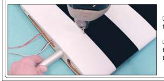
□ Slide one aluminum wing joiner tube into one outer wing panel until the tube bottoms out.
