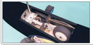
□ Install the retract assembly onto the landing gear mounting rails in the center fuselage pod, using the four large wood screws provided. The back edge of the retract mounting bracket should be 1-1/2" (38mm) behind the front bulkhead.
