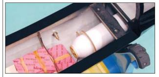
□ Install the air tank into the back of the center fuselage pod, using the plywood support provided.
