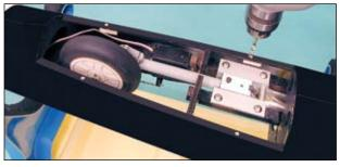
Glue one balsa block underneath each hinge mounting location on the two fuselage booms.
