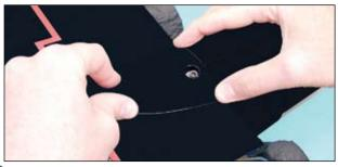
□ Glue the two rear fuselage boom fairings to the center wing panel, making sure not to get any glue between the center wing panel and the fuselage booms.
