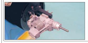
□ Install one engine mount assembly and one engine onto each fuselage boom, using the socket-cap screws, machine screws, washers and nuts provided. A four-stroke engine is shown. Installing a two-stroke engine will be the same.
