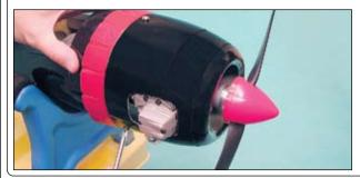
□ Install a remote fueling valve into each cowling to make it easy to fuel the airplane, then install the cowlings to the fuselage booms, using the six large wood screws provided.
