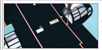
□ Plug the servo leads into your receiver and mount the center fuselage pod to the center wing panel, using the two longer socket-cap screws and two washers provided.
