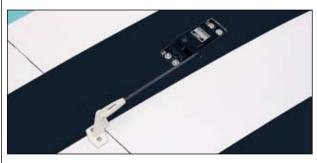
□ Install one flap servo into each wing panel. Each servo output shaft should be toward the trailing edge.
