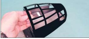
□ Cut out and install the rear window glass, using the same techniques that you used to cut out and install the forward window glass.
