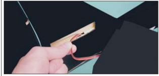
**IMPORTANT** You may need to adjust the size of the precut slot in the fuselage boom to prevent pinching the servo extension.
