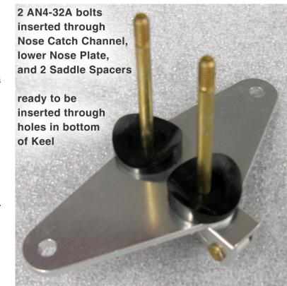
Photo: Attaching Top Nose Plate to Keel
