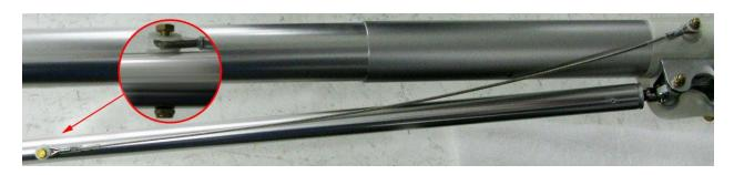
9. Attach the hardware for connecting the Cross Bar to the Channel Bracket. The Cross Bar will not be attached to this assembly until later, when the sail is added to the airframe. For now, attach the hardware so it can used later when needed to attach the Cross Bar.
