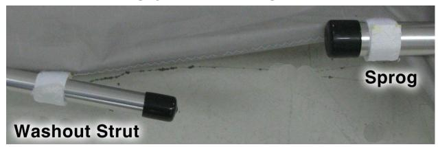
5. Pull the tip of the sail over the black cap at the end of the leading edges by pulling on the black strap, and be sure to set the yellow strap into the 1" wide slot at the end of the leading edge.
