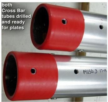
4. Prepare the center plates to be attached to cross bar tubes by using the Schematic Diagram labeled "Cross Bar Center Junctions" to arrange the layout of plates with bolts, half-spacers, washers, and Nylock nuts.
