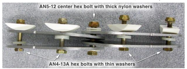
Photo: Side View of Center Cross Bar Plates with bolts, washers, and thin Nylock nuts
