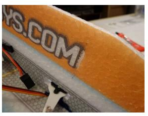
Apply Welders to the extreme ends of the cut out, where it captures the wood brace only. Leave the wider section in the middle free of glue for now.
