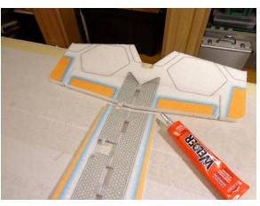
Locate the elevator/stab. Verify full down deflection is approx 50 degrees, carefully trim some foam from the bevel away if not. Apply glue via Tack Up Method
