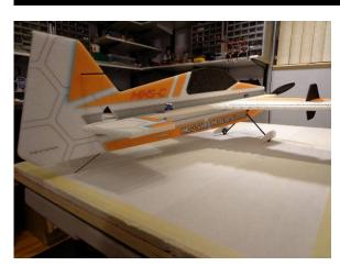
With the extra carbon rod from the Rudder, make a tail skid to protect the rear of the plane during ground operations
