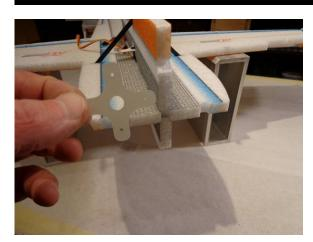
While the landing gear struts are drying, glue the fiberglass motor mount onto the front of the fuselage. Use the tack up method
