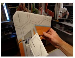
Glue the rudder on. Use the Tack up Method. Make sure it is in line and square with the vertical fuselage pieces
