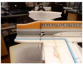
.... as well as the bottom edge of the wheel pants being parallel to the bottom edge of the fuselage
