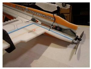
NOTE - This build was done with extensions on the rear servo side, ie Forward RX location. For Rearward RX location, the RX would be approx 1.0" behind the trailing edge of the aileron
