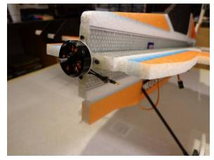
Secure the motor to the nose of the aircraft.
