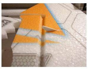
Glue the horn in. Flex the rudder back and forth to make sure the horn does not interfere. Hole in the horn should be in line with the hinge point
