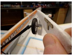
With the nozzle of the Welders tube, force some glue into the hole of the wood T-Brace, and apply a thin coat to the axle. Assemble the two pieces. Repeat for the other side
