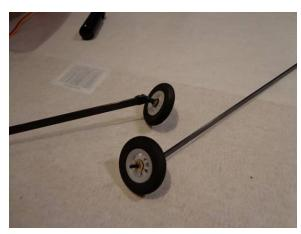
Drill the wheels out to fit the axles. Install and glue the inside washer then install the wheels. Install and glue the outside washer. Be Careful with the glue, wheels need to turn!
