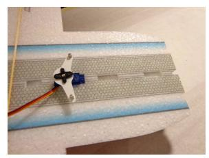
Install the aileron servo as shown. Note that the output shaft is to the REAR. Secure with a couple SMALL dabs of glue. Too much will make removal harder later if needed
