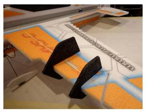
Attach the SFGs. Smaller ones outboard, and shorter side of both, down
