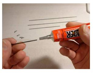
Put glue on pushrod by dipping it into the glue nozzle
