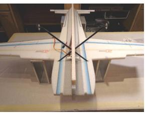
Flip back over so there is no pressure on the landing gear and allow to dry completely
