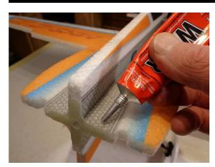
... first lay down a skim coat of Welders in all the area where the tape will be.
