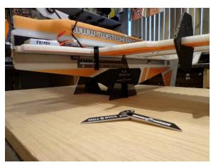
CG is 1.25" behind the spar or approx 3.56" from the leading edge of the wing.
