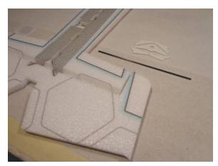
Locate the small rectangle carbon strip use to stiffen the elevator
