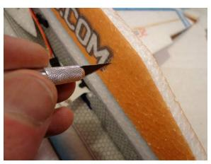
Next, install the landing gear onto fuselage, start by cutting out opening for legs and rectangular brace
