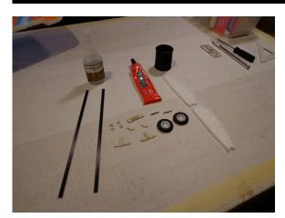
Prepare the Landing Gear. CA or Welders can be used. Wrapping with string will make it stronger. Remove all the tiny wood pieces from their plywood pack
