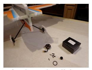
Locate the motor and assorted hardware. NOTE- if using 2s the included oring will work, but for extreme flying and 3s operation, the HD O-rings are recommended
