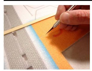
Cut out tabs that hold the wing and fuselage together so that the spar can be inserted
