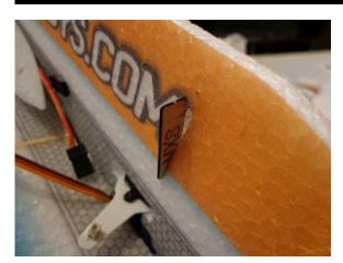
Slide the wood brace into the slot
