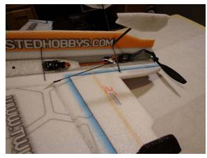
Mount the ESC as far back as possible. For rearward RX attach an extension long enough to the ESC that allows the RX to reach the rear servos
