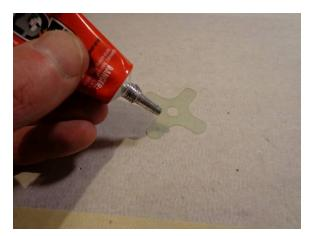
Apply glue to the mounts, install on nose, remove from nose, allow to tack up for approx. 5 minutes, assemble onto the airframe
