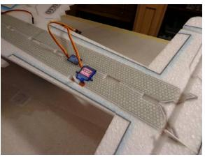
Install the rudder and elevator servos. NOTE - for extreme 3D control throws long servo arms are required. If not included in the servo hardware, fabricate by gluing on part of another horn. approx .75" is needed from center to link
