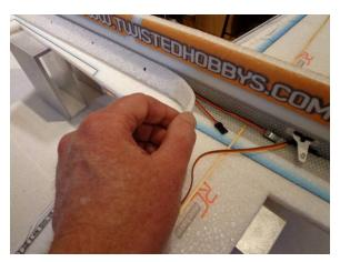
Carefully install the trusses. Make sure everything remains square. Leave one end free of glue until radio gear is installed.
