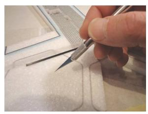
Locate the spar slot on the underside, cut deeper as needed. Test fit, spar should be flush with the underside of the elevator. Glue in, wipe away any extra glue
