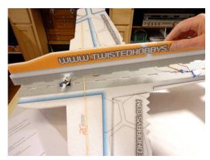
Install the lower fuselage. Use glue on full bottom surface and sides of tabs
