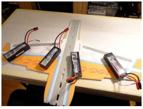
Weight down fuselage/wing/spar assembly on parchment paper, press together, let dry
