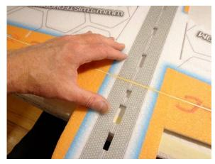
Insert spar, press fuselage/wing assembly together to ensure good glue joint on spar
