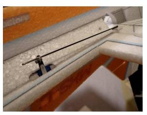
Install the Elevator Push Rod. Clip off any extra length.
