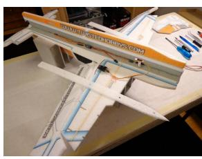
Install the trusses. Figure out first were you want to locate the RX and add servo extensions as required. NOTE- for rearward location only one extension on the ESC would be needed
