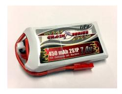
2 Cell / 450mAh / 5c Charge Rate Discharge 25c Constant / 50c Burst JST Connector / Dims. 65x29x11
