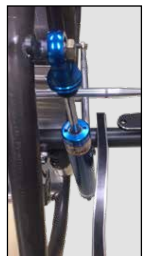
SHOCK INSTALL LEFT FRONT
