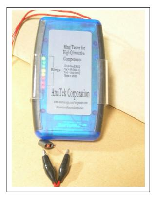
This ring tester is an inexpensive and effective way to test any high Q inductive component. It is especially useful for doing a quick check on flyback, line output transformers and other high frequency wound components like deflection yoke windings and SMPS transformers.
