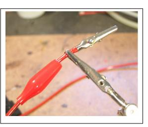
Strip approximately <sup>1</sup>/4" (4 mm) from the other end of the test leads, do not tin them. Push alligator clip insulators onto the leads first and then push the lead end into the center hole of the alligator clips as shown in the picture.
