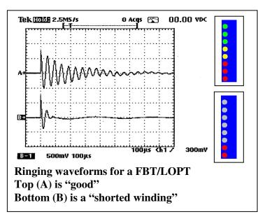
Waveform A shows the ring response to this tester's pulse for a good FBT/LOPT. Note several rings in a decaying fashion. This tester will count the rings that exceed its threshold and display them as lit LEDs as shown in the simulation to the right of waveform A.
