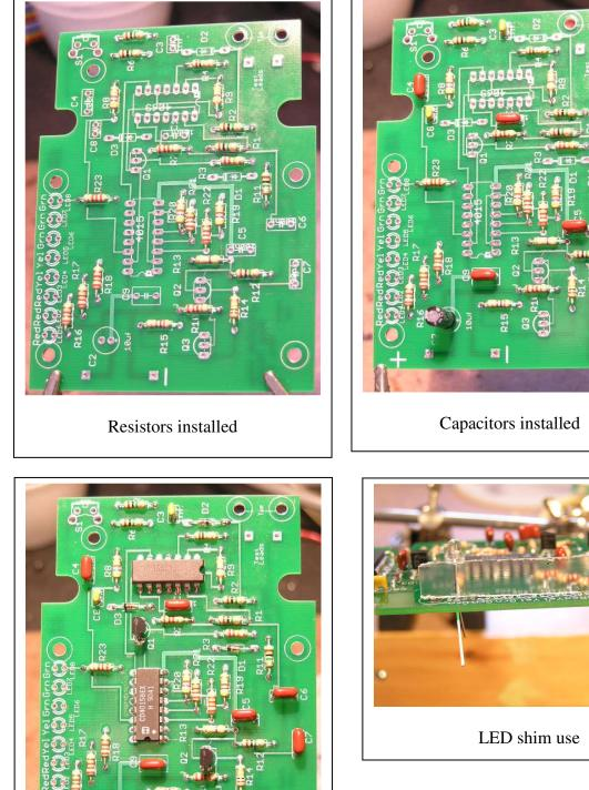
Semiconductors (not LEDs) installed
