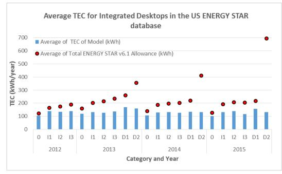
Figure 14 – Average TEC for Integrated Desktop Computers in the US ENERGY STAR database based on year first placed on the market against average ENERGY STAR v6.1 TEC allowance
