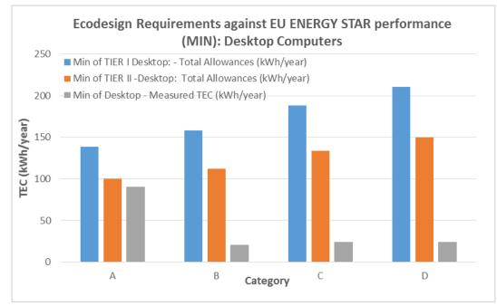
Figure 11– Minimum TEC for Desktop Computers in the EU ENERGY STAR database over time compared to the EU Ecodesign Requirements
