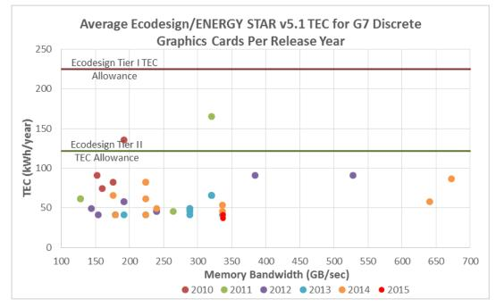
Figure 24 – Average TEC of High End Discrete GPUs per Year of Release Compared to the EU Ecodesign Allowances
