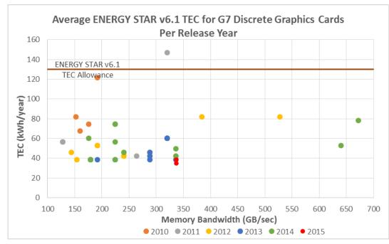
Figure 25 – Average ENERGY STAR v6.1 based TEC of High End Discrete GPUs per Year of Release Compared to the ENERGY STAR v6.1 allowances
