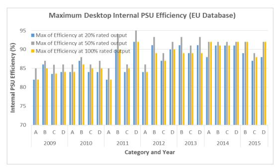
Figure 31– Maximum Internal PSU Efficiency at different loading points for Desktop Computers in the EU ENERGY STAR database
