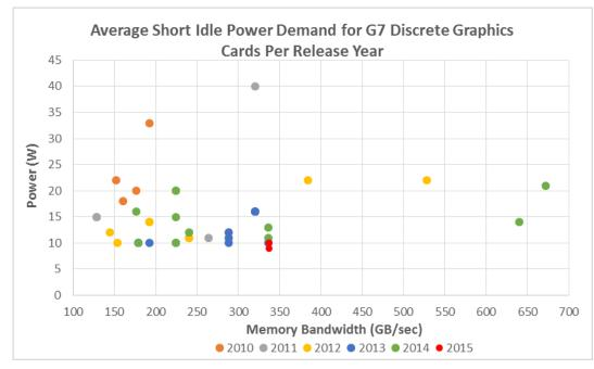
Figure 23 – Average Short Idle Power Demand in High End Discrete GPUs per Year of Release
