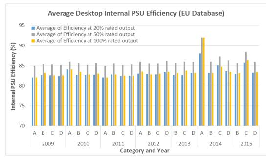
Figure 30 – Average Internal PSU Efficiency at different loading points for Desktop Computers in the EU ENERGY STAR database
