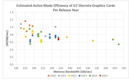
Figure 28 – Estimated Active Mode Efficiency of High End Discrete GPUs per Year of Release
