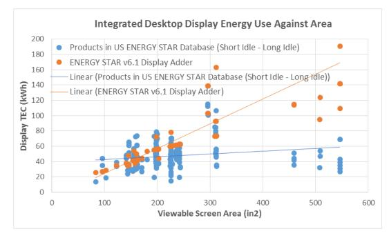
Figure 7 – Estimated ENERGY STAR v6.1 TEC of Displays and Allowances in Integrated Desktop Computers Listed in the US ENERGY STAR database (May 2015) against Viewable Screen Area
