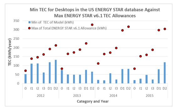
Figure 16 – Minimum TEC found for Desktop Computers in the US ENERGY STAR database based on year first placed on the market against the maximum ENERGY STAR v6.1 TEC allowance found
