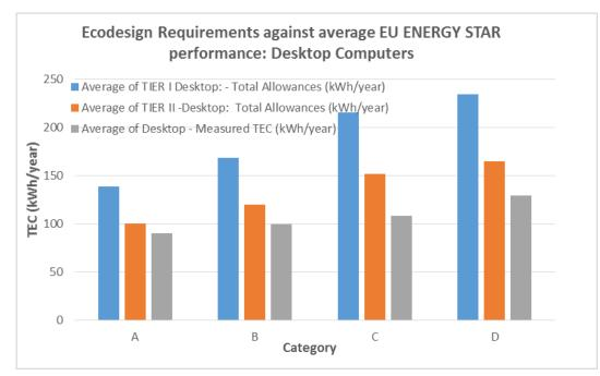
Figure 9 – Average TEC for Desktop Computers in the EU ENERGY STAR database over time compared to the EU Ecodesign Requirements
