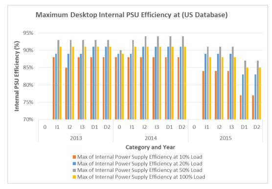
Figure 33 – Maximum Internal PSU Efficiency and loading for Desktop Computers in the US ENERGY STAR database
