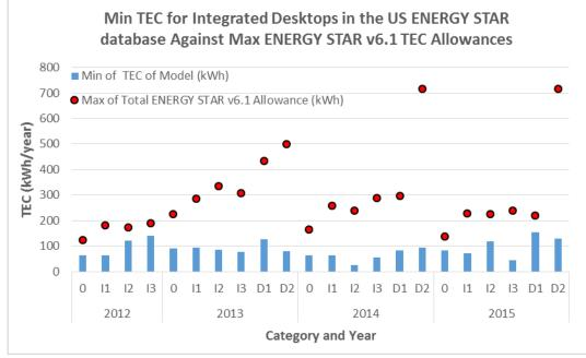
Figure 17 – Minimum TEC found for Integrated Desktop Computers in the US ENERGY STAR database based on year first placed on the market against the maximum ENERGY STAR v6.1 TEC allowance found
