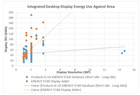
Figure 37 – Estimated ENERGY STAR v6.1 TEC of Displays and Allowances in Integrated Desktop Computers Listed in the US ENERGY STAR database (May 2015) against Resolution
