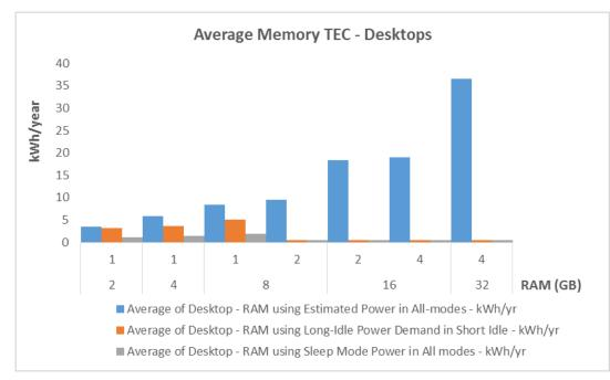
Figure 40 – Average Desktop based TEC for Sample RAM Modules
