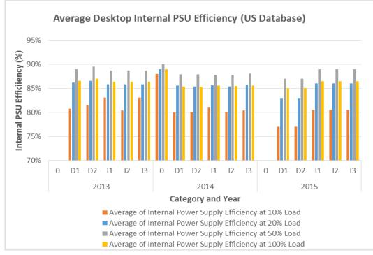
Figure 32 – Average Internal PSU Efficiency and loading for Desktop Computers in the US ENERGY STAR database
