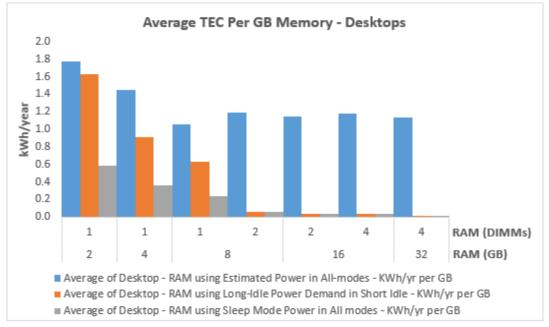
Figure 38 – Average Desktop based TEC per GB of RAM for Sample RAM Modules
