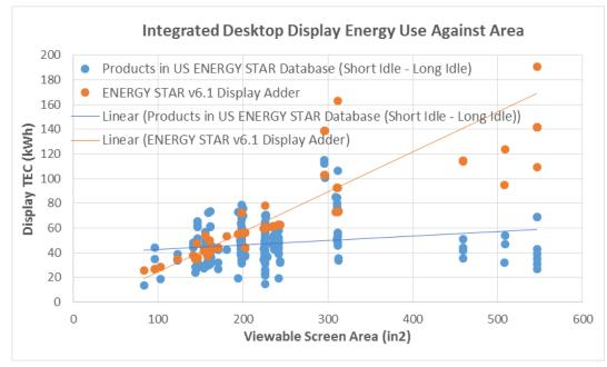
Figure 36 – Estimated ENERGY STAR v6.1 TEC of Displays and Allowances in Integrated Desktop Computers Listed in the US ENERGY STAR database (May 2015) against Viewable Screen Area
