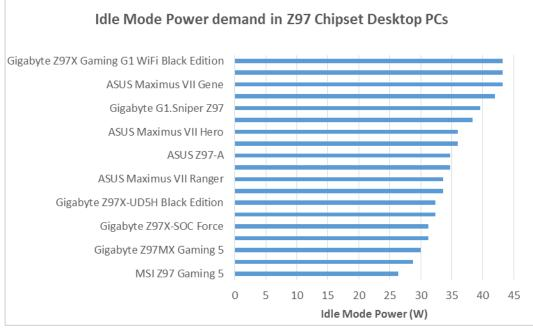
Figure 22 – Idle Mode Power demand of Z97 Chipset Motherboards<sup>7</sup>
