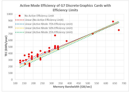
Figure 29 – Impact of Active Mode Efficiency Requirements on TEC of High End Discrete GPUs
