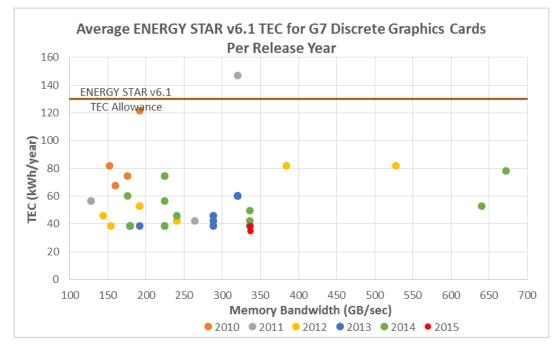
Figure 6 – Average ENERGY STAR v6.1 based TEC of High End Discrete GPUs per Year of Release Compared to the ENERGY STAR v6.1 allowances
