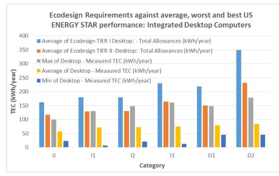
Figure 20 – Average EU Ecodesign Regulation TEC requirements for Integrated Desktop Computers in the US ENERGY STAR database against average, maximum and minimum TEC values
