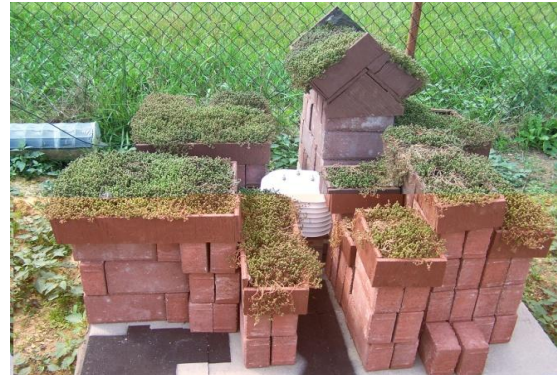
Figure 15. Green Roof Hardware Scale Model.
