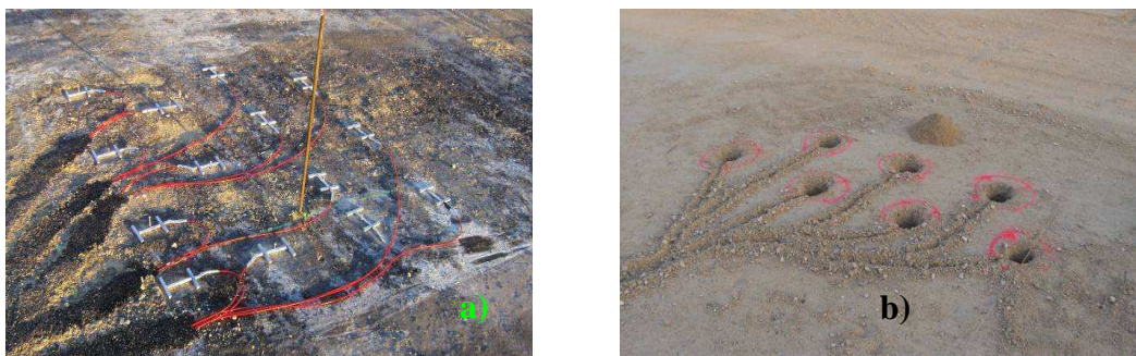
Figure 13 a - Mesh of horizontal X and Y strain sensors (base of the asphalt layer), b - Mesh of vertical strain sensors (untreated materials), after [Broutin et al., 2008]
