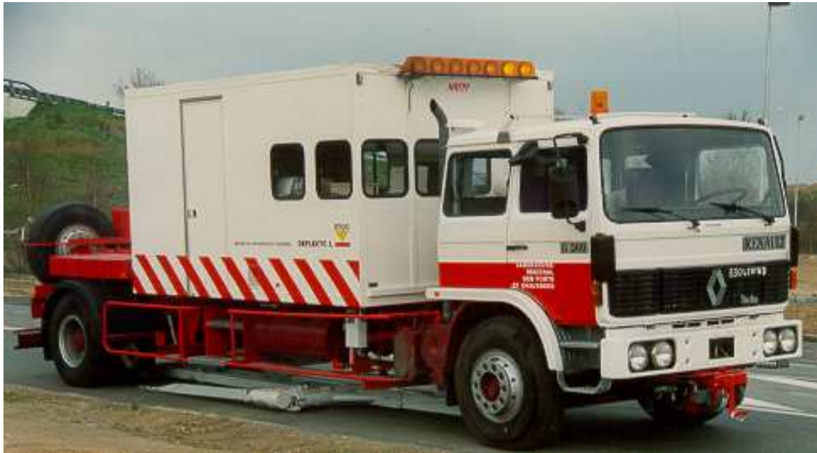
Fig. 0-15 The Lacroix Deflectograph (source: LCPC's database)
