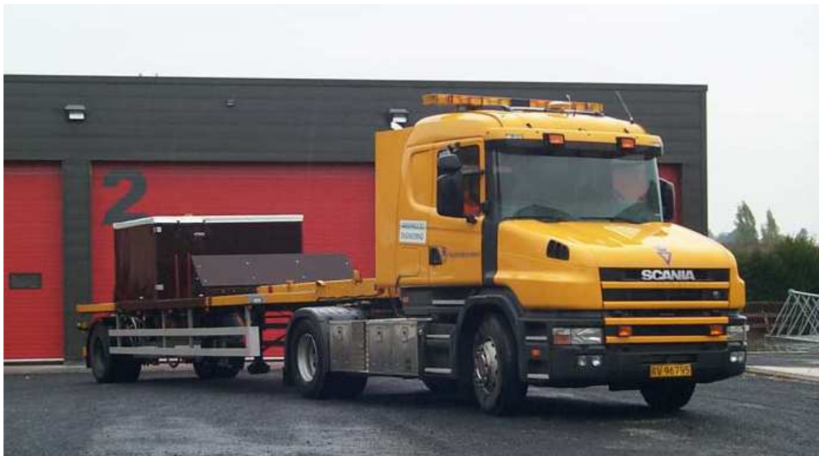
Fig. 0-19 Traffic Speed Deflectometer (TSD) on the LCPC's Nantes site in 2003, after J.M. Simonin, French "Assessment of the Road Deflection Tester in France" report, [FORMAT, 2005]
