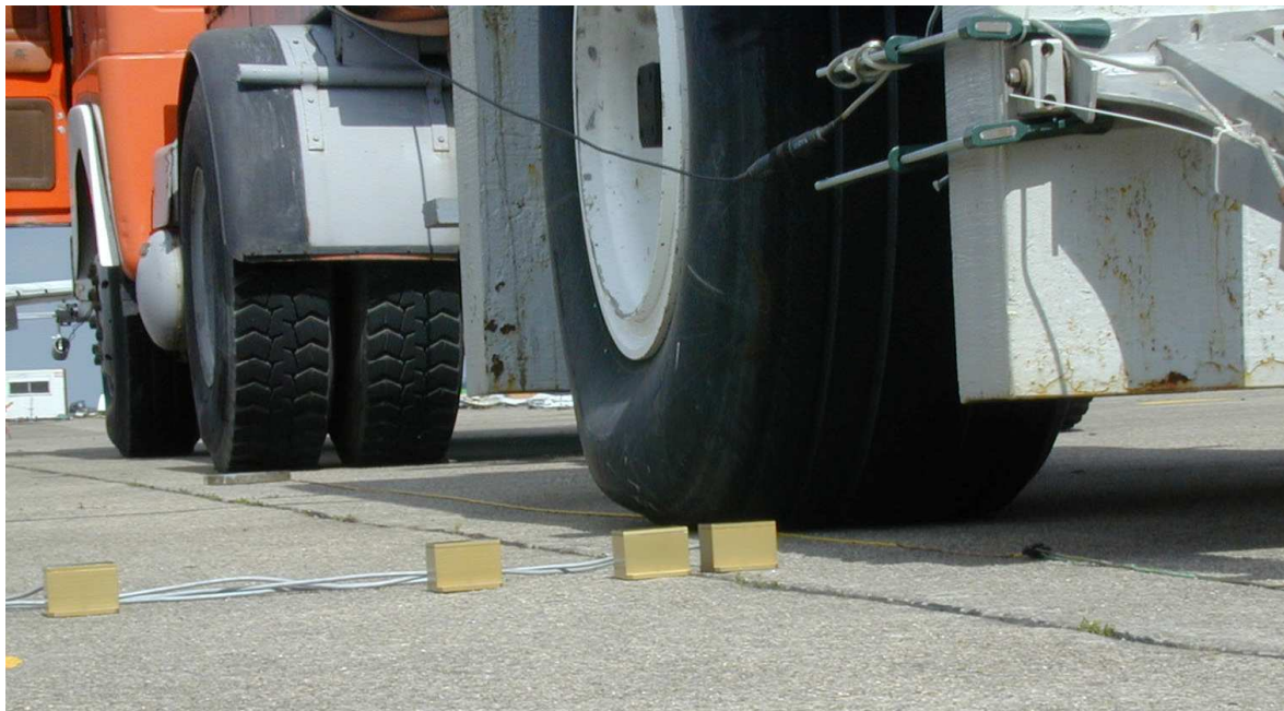
Fig. 0-14 STAC's inclinometer system, zoom view (Photograph by D. Guédon, Toulouse LRPC)
