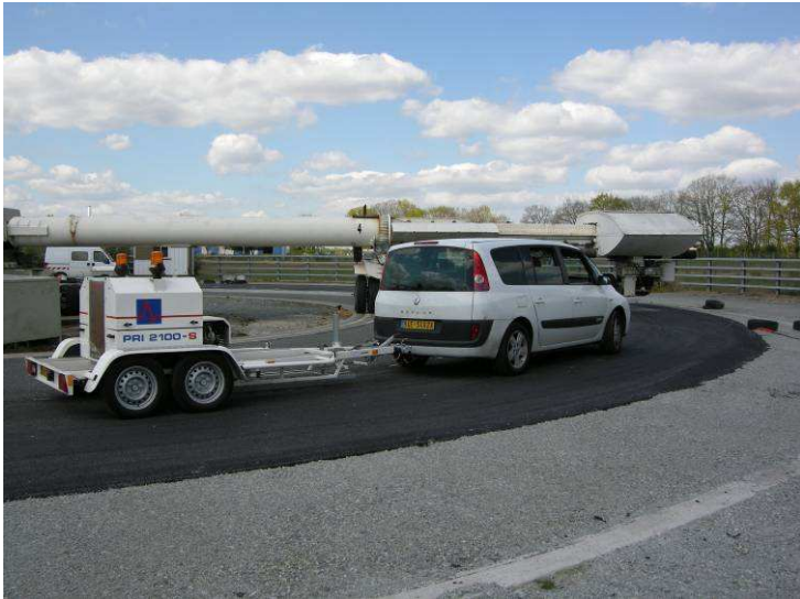
Fig. 3-2 HWD test on the LCPC’s fatigue carrousel test facility (photograph by M Broutin)
