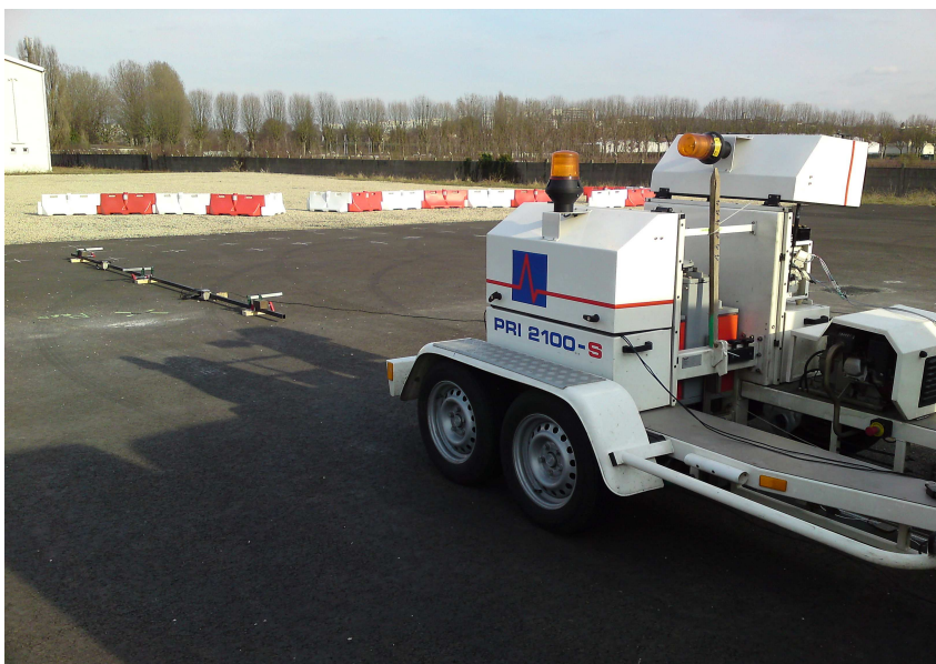
Fig. 1-43 Test setup to measure long radial distances deflections
