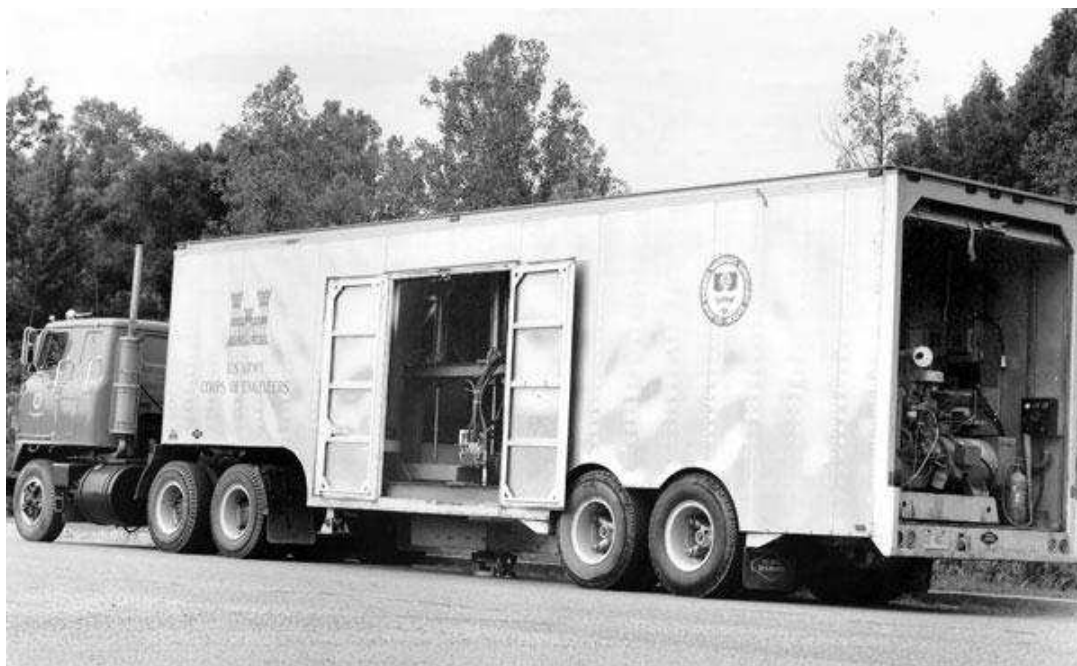
Fig.0-17 The WES 16-kip Vibrator; sources: US army website ( http://gsl.erdc.usace.army.mil/gsl-history/Chap7.html )
