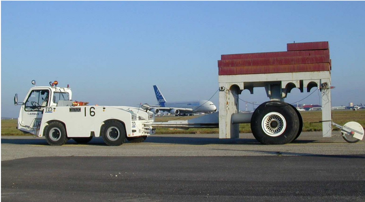
Fig. 0-13 STAC's A 340 two-wheel landing gear loaded at 25 tons (250 kN) per wheel here trailed by the Airbus truck on the HTPT test facility (Photograph by D. Guédon, Toulouse LRPC)
