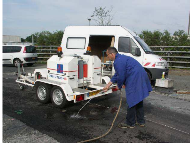
Fig. 3-4 Continuous spraying of the surface pavement during the whole tests series duration (Photograph by M. Broutin)
