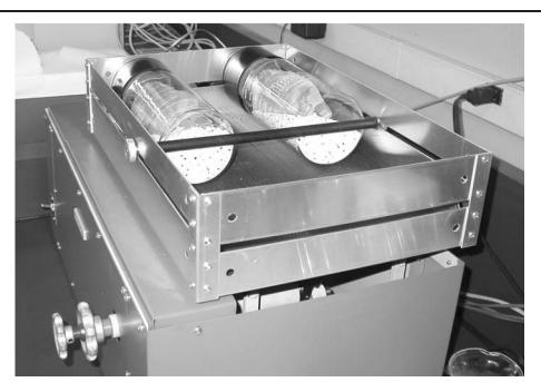
FIGURE 2. Exam glove durability test setup
