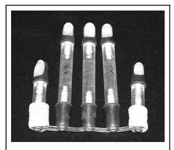
**FIGURE 1.** Top view of an assembled hand phantom with artificial fingernails applied to the rubber stoppers
