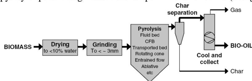
**Figure 12:** Schematic of a fast pyrolysis process (Bridgwater, 2006)
