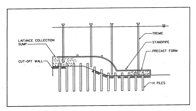
Figure 2. Tremie concreting into precast concrete form
