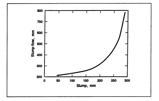
Figure 8. Slump versus slump flow
