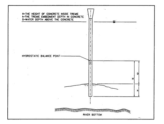
Figure 14. Hydrostatic balance point in a tremie system
