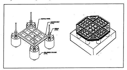
Figure 11. Configuration of the three intake velocity caps
