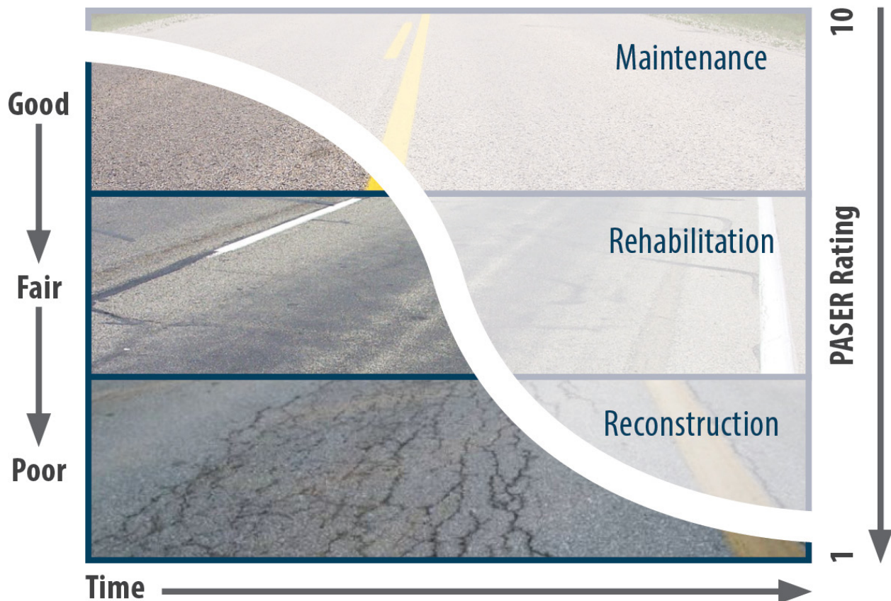
Figure 9-1 Example of progression of deterioration from good to poor. Source: Asset Management Guide, Indiana LTAP (June 2017)
