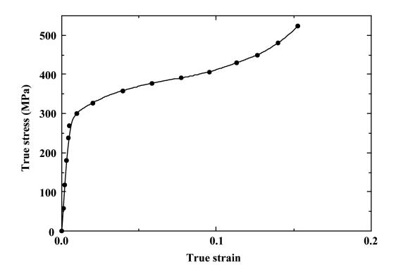
6.44 The following true stresses produce the corresponding true plastic strains for a brass alloy:
