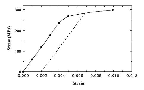
(b) The elastic modulus is the slope in the linear elastic region (Equation 6.10) as
