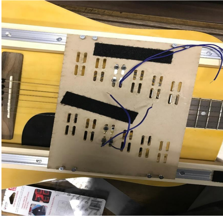
Figure 44: Mounting Plate Top View with Solenoid Pair
