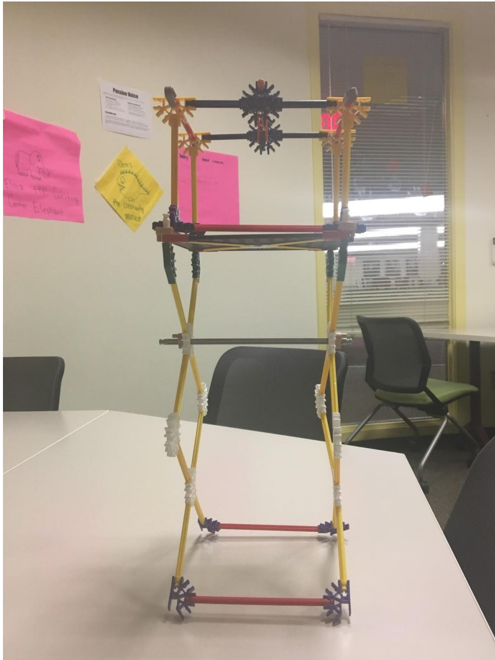
Figure 24: Zero Order Prototype of Scissor Lift Support for Design Concept 1
