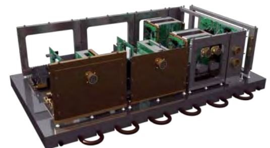
Cut away of NASA 300V PPU
