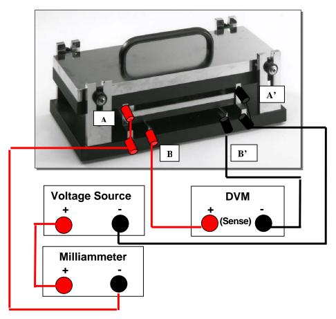
Figure 1.0-2: Model 831 meter connections
