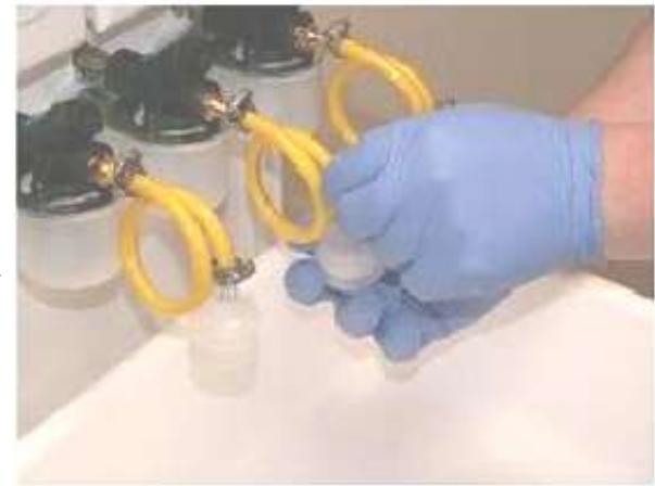
Use Air Pump to Aid Drying (2-45 minutes)
