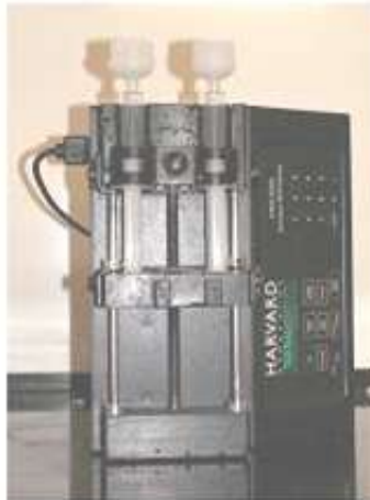
Use Syringe Pump to Force Sample through Device (3 minutes)
