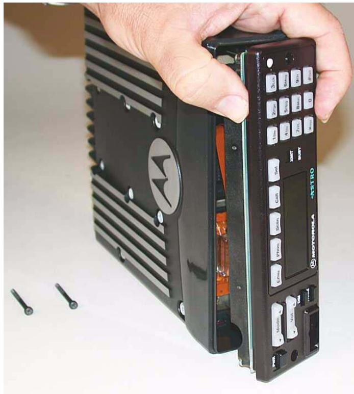
Figure 8-4. Removing the Control Head
