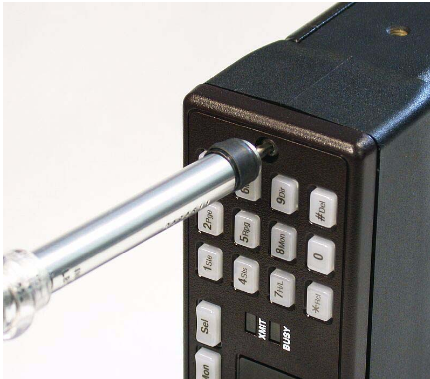
Figure 8-3. Removing the Front Panel Screws
