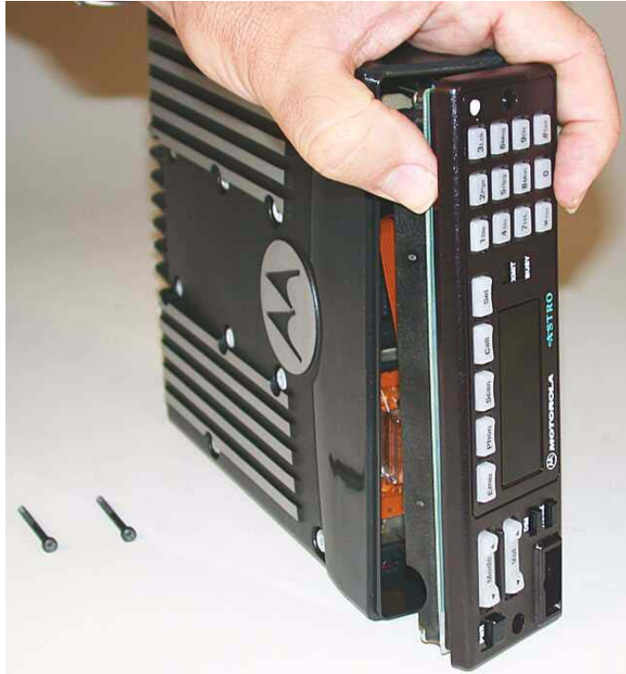
Figure 8-36. Inserting the Control Head Into the Transceiver
