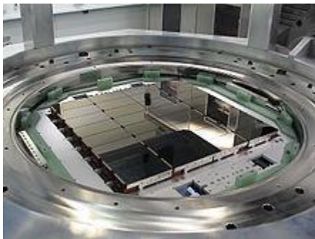
The OmegaCAM camera lies at the heart of the VST. This view shows its 32 CCD detectors that together create 268-megapixel images.
