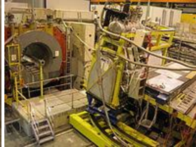
Beamline from SPS feeding 20 GeV positrons to AMS for alignment testing at the time of the picture.
