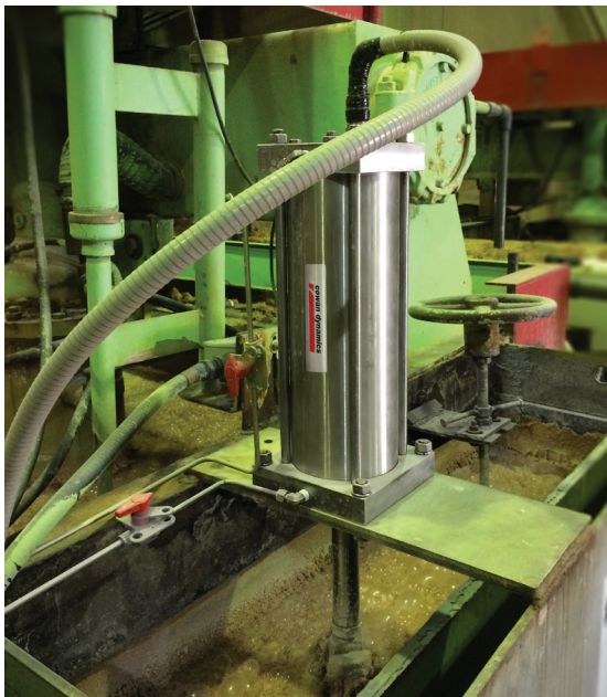
Stainless Steel AT Series with remote positioner in a potash plant
