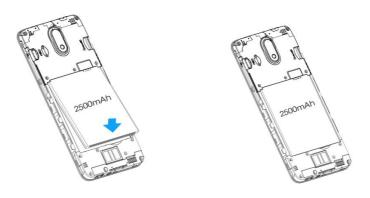
Align the contacts of the battery with the contacts in the phone and gently press the battery down into place.
