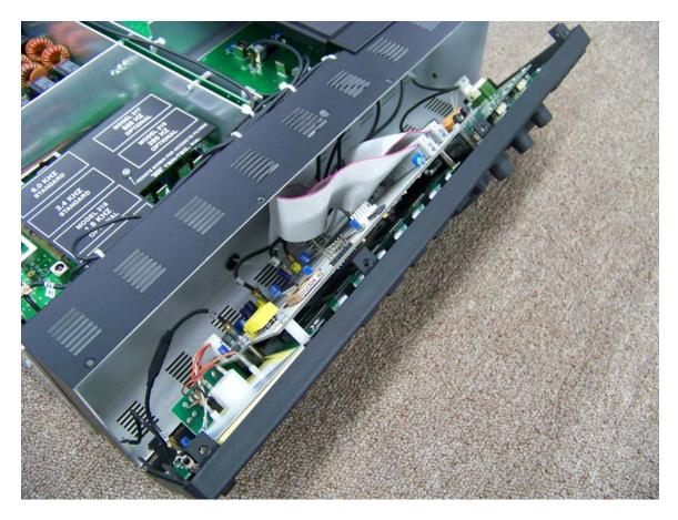
2. Turn the transceiver right side up. Around the perimeter of the front panel of the transceiver will be 12 Philips screws inserted in plastic tabs. Remove all 12 screws. VERY CAREFULLY AND **SLOWLY** pull the front panel forward and tilt as shown.
