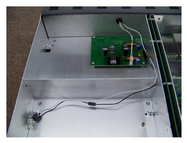
4. Re-attach the front panel to the transceiver chassis with the 12 Philips screws removed in step 2. Turn the transceiver upside down with the rear of the radio facing you. Route the cable attached to the front panel in steps 1-3 through the notch in the chassis shown at the right of this picture. The other end will be attached to the automatic antenna tuner circuit board in a later step.
