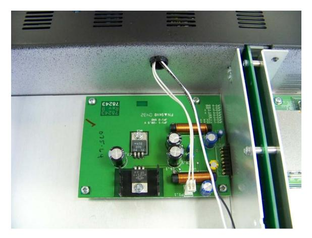
1. Remove rig covers. Turn the transceiver upside down with the rear of the radio facing you. Near the center of the rig is a small circuit board with a white cable fed through a plastic grommet towards the front panel. One of the cables provided with the kit has one white wire and one black wire and two connectors marked "11" and "T". Take the end of the cable with the connector marked "11" and push the connector through the plastic grommet as shown in this illustration.
