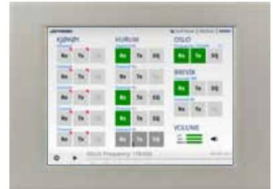
Delivered with 8.4" touch screen panel for panel mounting, stereo speakers and handheld microphone
