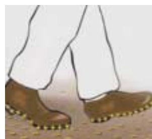
Non-conductive soles or floor covering increase static charge.
