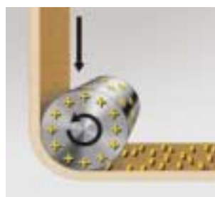
Roller used to roll off foil.
