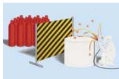
Small smoldering solid particles that are produced during welding and scattered.
