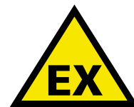
Warning sign for places where explosive atmospheres may occur.
