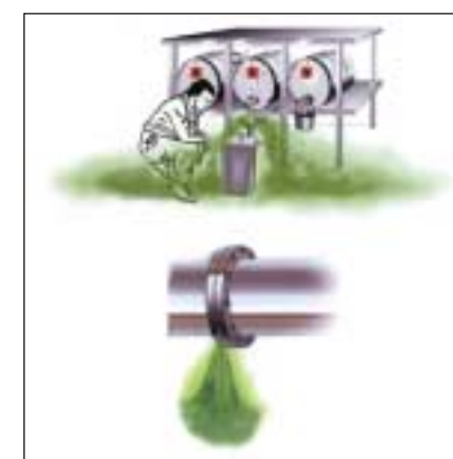
Examples of the rise of explosive atmospheres during filling and transport processes of gases and liquids.
