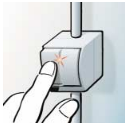
Sparking when pressing a light switch.
