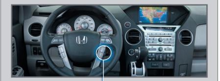
While on the Trip Computer display, press the SEL/RESET button to access trip information. Press either Info (▲/▼) button to toggle through the various screens, or the SEL/RESET button for sub-displays.
