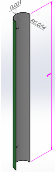
Figure 23. Isometric View of the Blade (Units in Meters)
