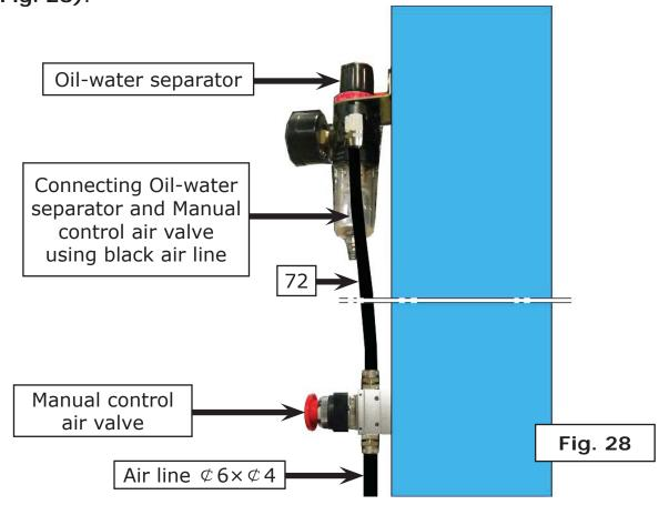
5. Connecting air inlet (Air supply pressure 5kg/cm2- 8kg/cm2), adjusting the air pressure of Oil-water separator to 0.4 - 0.6MPa (See Fig. 29).
