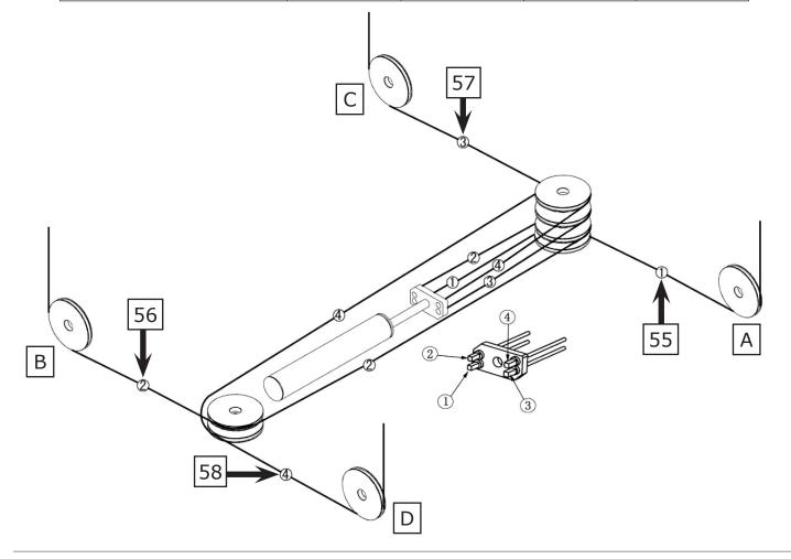
2. The cable pass through the cross beam to top plate of columns and be screwed with cable nuts (See Fig. 22).
