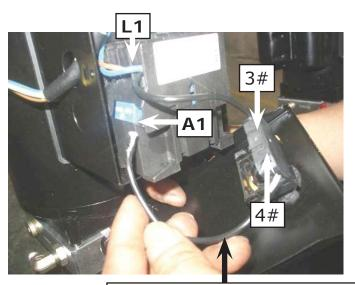
Fig. 35 Remove this line before connecting the Limit Switch
