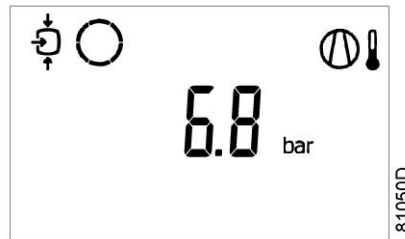
Main screen with shutdown indication, element outlet temperature
