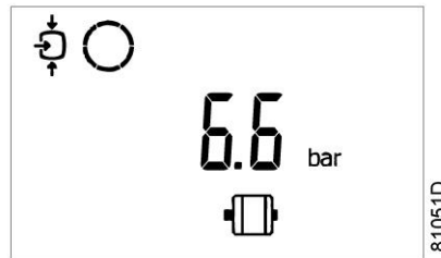
Main screen with shutdown indication
